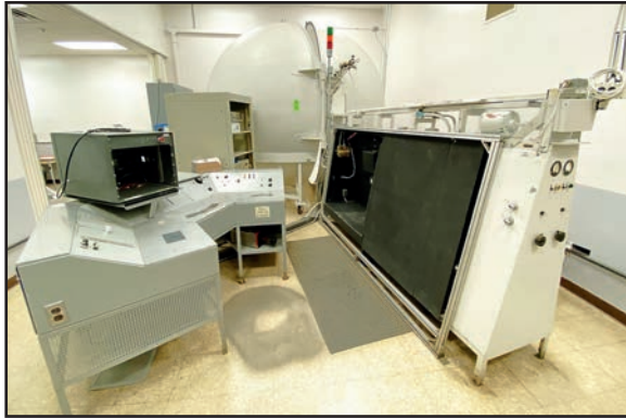
8' DIAMETER LUMENS SPHERE FOR LIGHT OUTPUT TEST SYSTEM, W/ HP 6030A SYSTEM POWER SUPPLY, SPITZENBERGER SPIES EV 1200/FS POWER AMPLIFIER AND NT 1200 POWER SUPPLY, INVERTRON LC-1201B DYNAMIC LINE CORRECTOR, AND CONTROL CABINET
