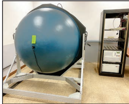
5' DIAMETER LUMENS SPHERE FOR LIGHT OUTPUT TEST SYSTEM, W/ SPITZENBERGER SPIES EV 1200/FS POWER AMPLIFIER AND NT 1200 POWER SUPPLY
